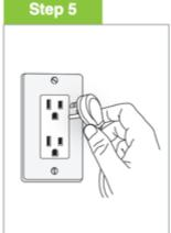
Plug the power strip into a grounded outlet receptacle. The ground and surge lights on the power strip will illuminate indicating the that power strip is properly grounded, and that surge protection is active.
