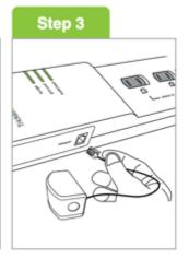
Plug the SensorClick motion sensor into the port on the side of the power strip that looks like a phone jack and is marked "sensor".
